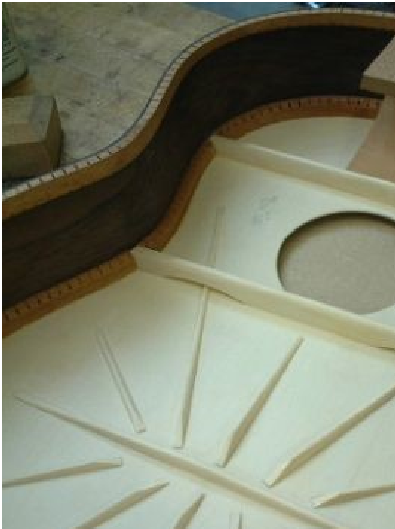
(5) Principle of radial Bracing used in particular by Humphrey for his first guitars "Millenium".
