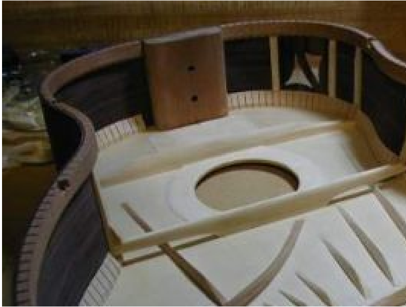
(4) Asymmetric Bracing imagined by the Dr.Kasha in the 1970s to increase its effectiveness. The great complexity of its realization under the actual results obtained was right of him. It is much more used by the last square of its defenders across the Atlantic.
