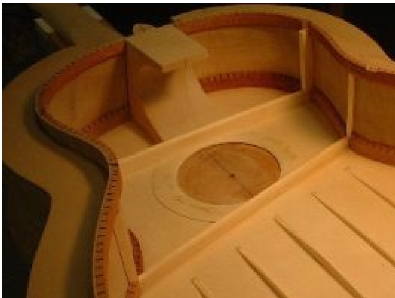
(3) Bracing "parallel" to the grain and crossbar oblique (Hernandez y Aguado). This Bracing increases the sensitivity of the top by relaxing. Dipping the acute bar to control the response in the top of the spectrum.
