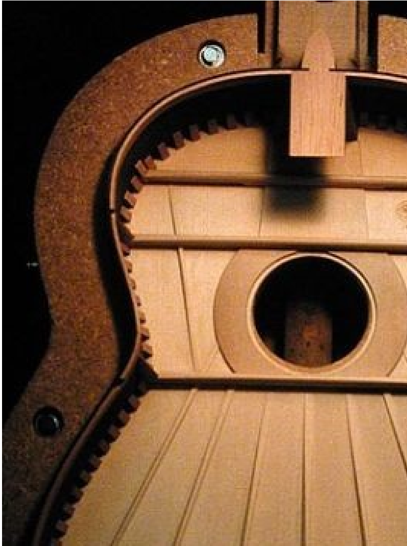
(1A) Evolution modern in the previous schema by opening passages in lower harmonic bar and add a plate of reinforcement under the bridge.
