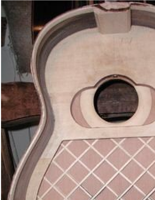
(6) The Smallman Bracing. An imposing framework supports an ultra-slim top of which the lower part is with trellis composite wood / balsa or graphite.
